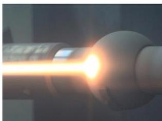
One of the main focus for the manufacturer JDV Valves Ltd. are on the well known « HVOF »-process. The principle behind this is a combination of plasma and detonation processes for surface coating with cobalt-chromium compounds. Depending on the requirement, specific hardnesses can be achieved up to 70 HRC.
